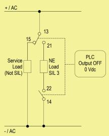
Contacts 13-21 and 14-22: the SIL 3 Safety Function is met when the relays are de-energized, contacts are open, NE load is de-energized.
