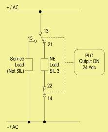
Contacts 13-21 and 14-22: in normal operation relays are energized, contacts are closed, NE load is energized.
